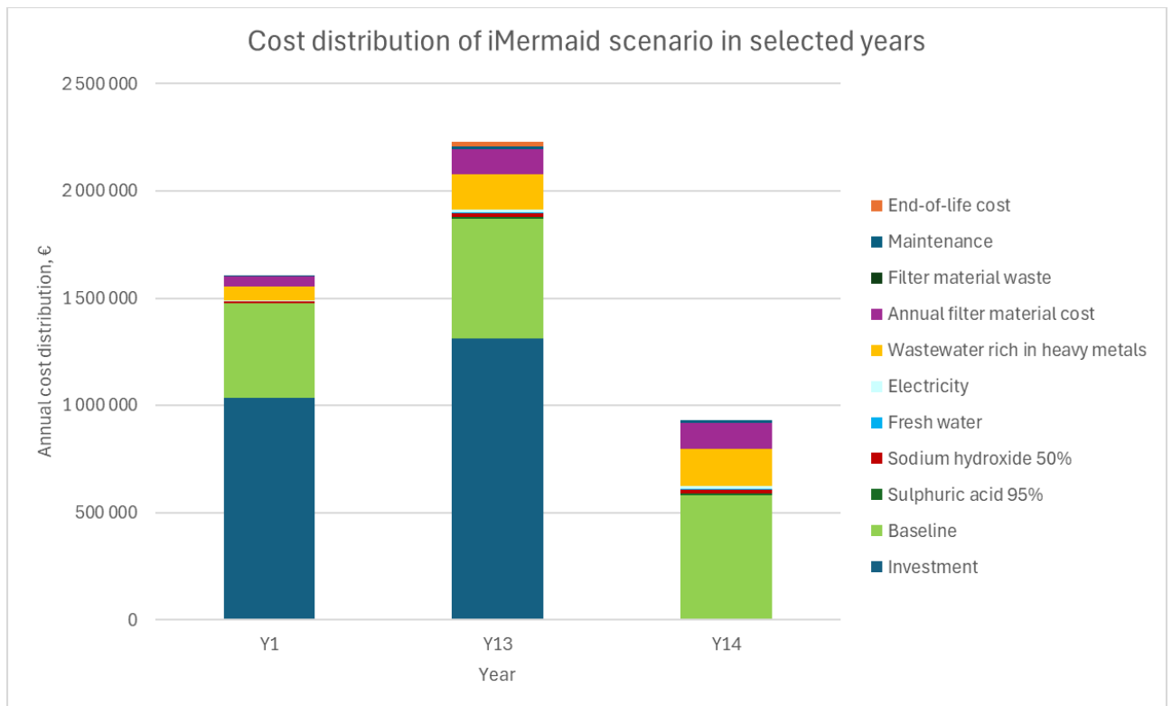
Figure 12: Annual direct cost distribution for selected years in the 20-year analysis period for Use Case 3 iMERMAID scenario (considering annual 2% inflation).
