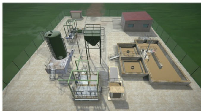
Figure 2: A snapshot of the immersive Digital Twin - San Esteban de Litera Wastewater Treatment Plant.
