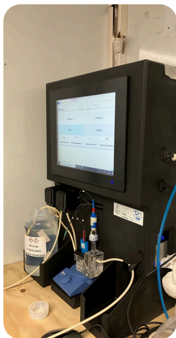
Figure 1: The HMBox working at the WWTP in Brandizzo (Turin, Italy).
