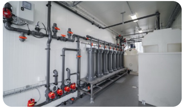
Figure 2: Picture of a 4D Scavenger unit designed for heavy metal removal from industrial wastewater. Picture shows the 4D Scavengers modules (8 pieces) as well as process piping and equipment.
